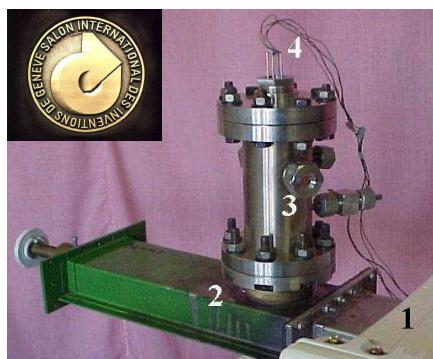
Fig.6. Microwaves cavity for heating lossless material [6] (nonpolar solvents)
