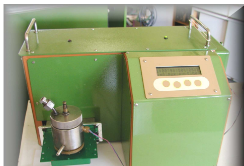
Fig. 7. Microwave unit for chemical treatments with microcontroller and RS232 PC interface
