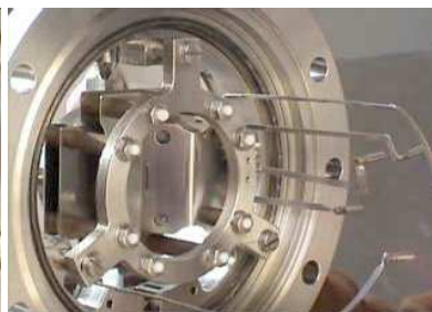
Fig. 3. The multifunctional detector mounted in the spectrometric tube of the SMIT-1 apparatus.
