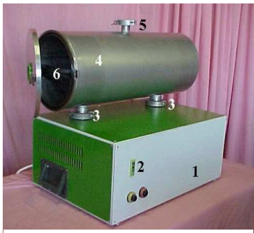
Fig. 5. Microwave plasma unit for surface activation
