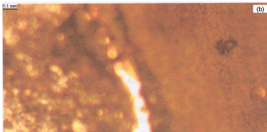
Fig. 4. Microstructure of a welded dental stainless steel. In the upper right corners is the stainless steel and the rest of images shows the weld material.
