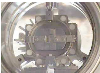
Fig. 2. The adjustable slit mounted in front of the detector.
