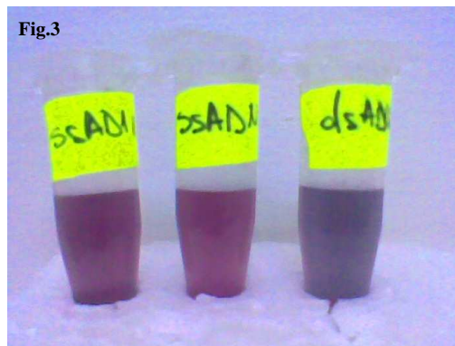
Fig. 3. Photographic image of gold colloid mixtures with (from left to right): ssDNA, ssDNAc and dsDNA in which NaCl solution was introduced.
