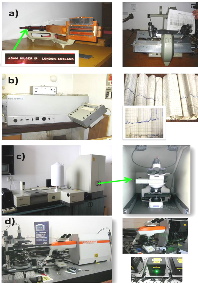
Fig. 3. Four generations of Raman spectroscopy equipment at Babes-Bolyai University: a) Hilger spectrograph (left) with the constant deviation quartz prism; Abbe comparator (right) allowing to read the wavelength by comparison with the positions of the iron reference spectral atlas; They were used in the period from 1933 to early '70-ths; b) Double grating GDM 1000 monochromator with photomultiplier as detection system and XY stage for spectra recording on paper rolls (used between 1970-1998); c) FT-IR, FT-Raman & micro-Raman Bruker equipment (since 2002, still running); d) Confocal Renishaw InVia Reflex Raman microscope coupled with the NT-MDT Ntegra Spectra SPM microscope; 5 lasers with 6 available lines, 325,442, 532, 633, 785 and 830 nm respectively, spectral resolution 0.5\text{ cm}^{-1} in visible and 1\text{ cm}^{-1} in UV and NIR (since 2013).
