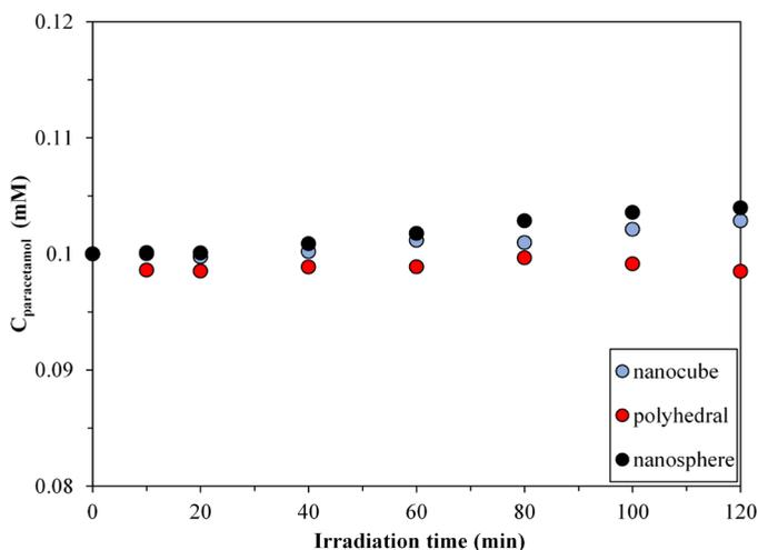
**Fig 8:** The photocatalytic degradation of paracetamol using nanomaterials: nanocube (blue dots), polyhedral (red dots), and nanosphere (black dots) (due to the small amount of material the 30- and 50-minutes sample was not taken).
