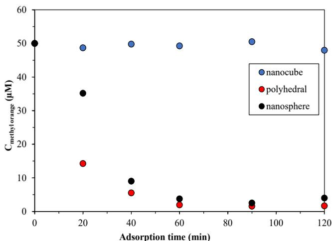
**Fig 5:** The MO adsorption test of differently shaped CeO<sub>2</sub> nanomaterials: nanocube (blue dots), polyhedral (red dots), and nanosphere (black dots).
