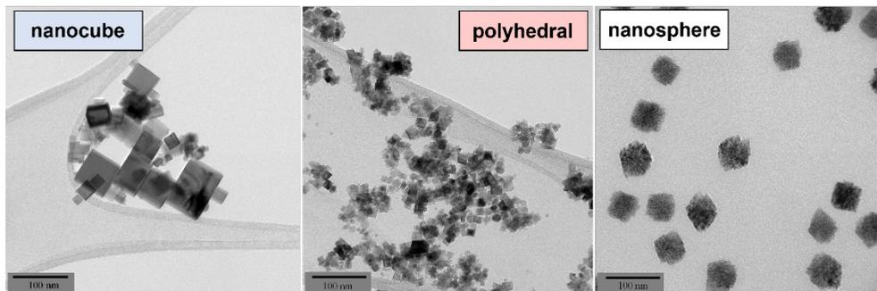
**Fig. 2:** Transmission electron micrographs of differently shaped CeO<sub>2</sub> nanomaterials: nanocube ( $\bar{d}$ ~25 nm), polyhedral shaped ( $\bar{d}$ ~15 nm), and nanosphere ( $\bar{d}$ ~60 nm).
