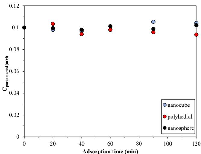
**Fig. 6:** The paracetamol adsorption of differently shaped CeO<sub>2</sub> nanomaterials: nanocube (blue dots), polyhedral (red dots), and nanosphere (black dots).
