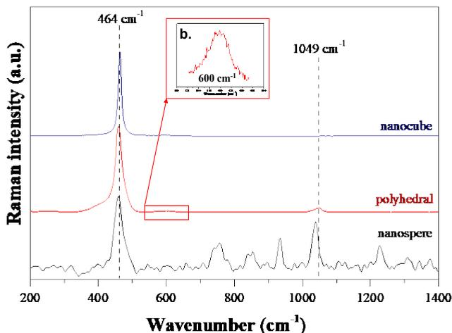
**Fig. 3:** The Raman spectra for differently shaped CeO<sub>2</sub> nanomaterials: nanocube (blue line), polyhedral (red line), and nanosphere (black line): entire graphs (a) and inserted graph - magnified (b)
