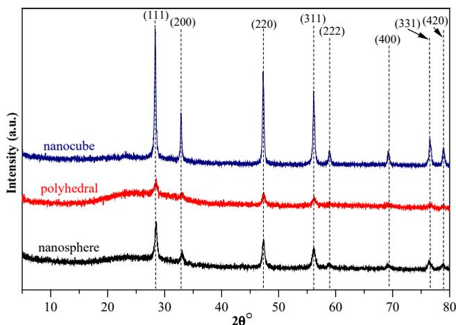
**Fig. 1:** The XRD patterns of differently shaped CeO<sub>2</sub> nanomaterials: nanocube (blue line), polyhedral (red line), and nanosphere (black line)
