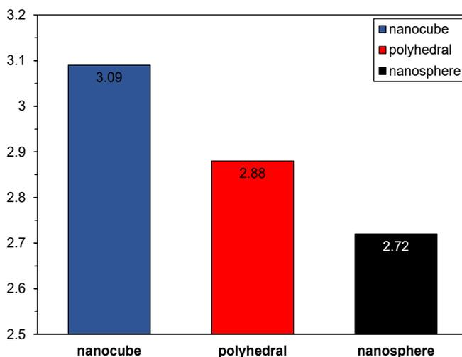
**Fig. 4:** The estimated bandgap energy values calculated by Kubelka Munk equation for the CeO<sub>2</sub> nanomaterials: nanocube, polyhedral, and nanosphere.
