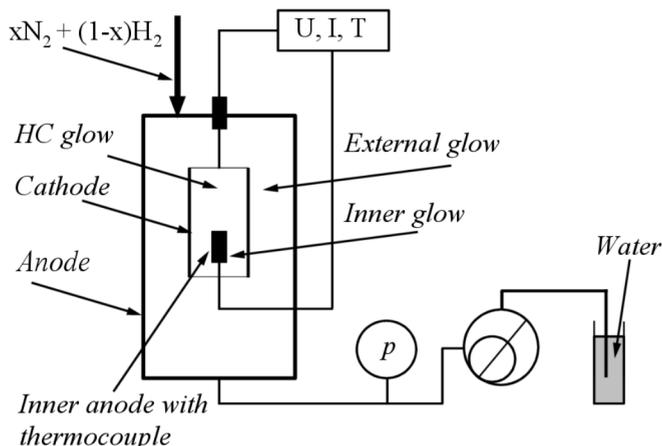
**Fig. 1.** The diagram of the experimental equipment
