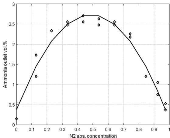
**Fig. 3.** Formation of ammonia from different gas mixture –  $xN_2+(1-x)H_2$ .
