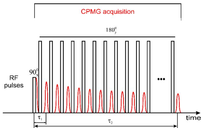
**Fig. 1.** The CPMG pulse sequence used for the  $^1\text{H}$  NMR data acquisition.
