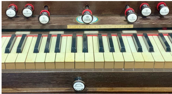
Keyboard and stops of the Harmoniphrase; the lower register activates the automatic system. 10
