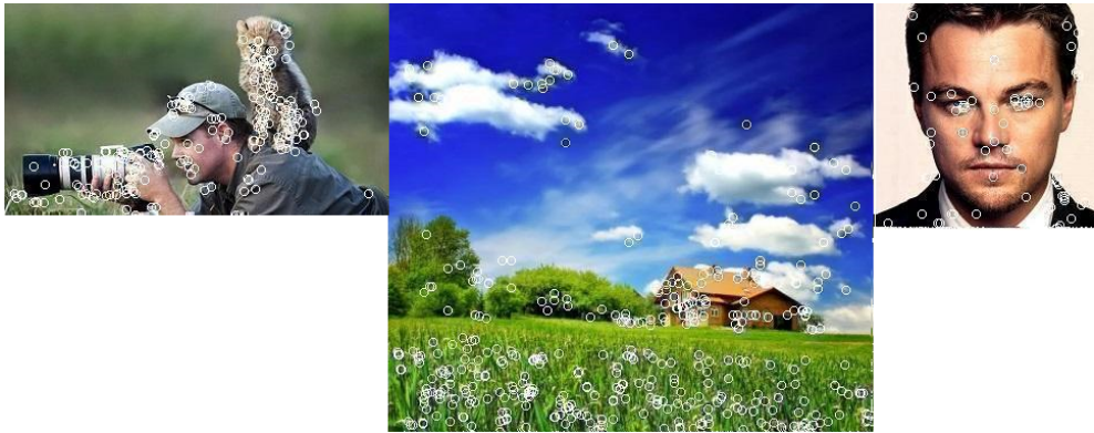
FIGURE 14. The final set of keypoints detected in our test images using SIFT-FAST approach (after low-contrast filtering, interpolation)
