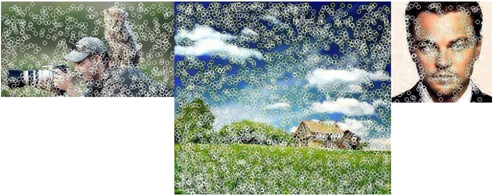
FIGURE 11. The first set of keypoints detected in our test images using classical SIFT.
