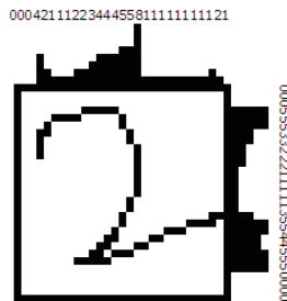
FIGURE 1. Histograms for digit 2. For each row and column we have counted the ink pixels.
