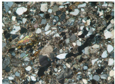
Fig. 8. Microscope analysis in plane – polarized light. Fig. 9. Microscope analysis in crossed – polarized light. Both photos show: mica, quartz and bioclast fragments.
