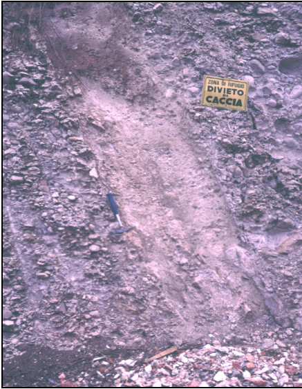
Fig. 1. Example of Quaternary active fault at the Alpine margin (S. Ambrogio din Valpolicella, west of Verona, northern Italy): band of cataclasites in Pliocene-Lower Pleistocene conglomerates. For details on this fault see Castaldini et al (1988).
