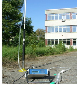
Fig. 2. The NDIR, used for the CO 2 determination.
