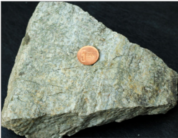
Fig. 5 – Porphyroid gneiss of Pietrosul Bistriței, found on the Neagra Broștenilor valley (July 2009).
