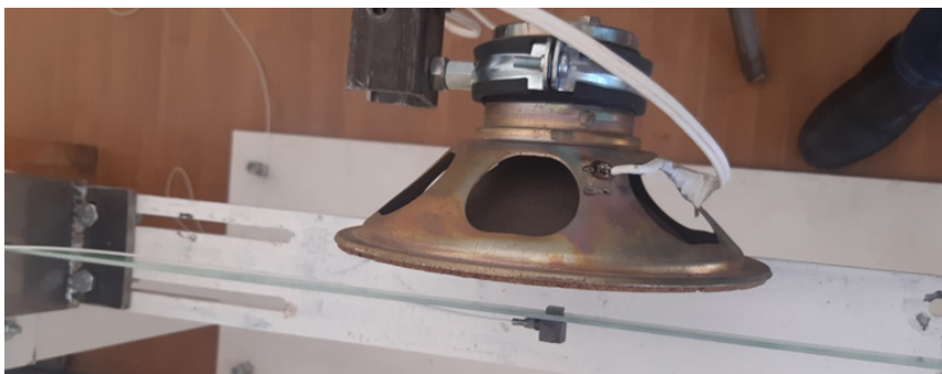
Figure 3. The beam with accelerometer and weight and the excitation system (upper view)
