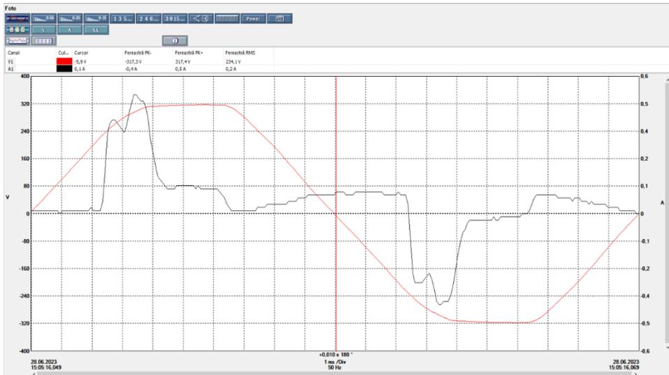
**Figure 7.** Voltage and current waveforms in operation of a toroidal fluorescent lighting source.
