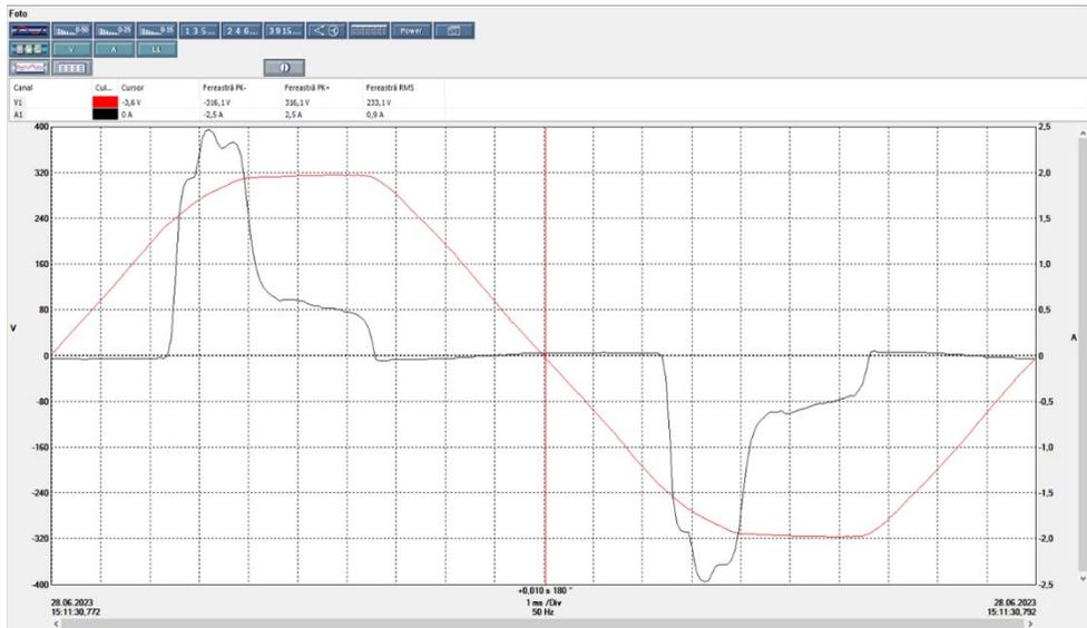
**Figure 9.** Voltage and current waveforms when operating with all bulbs on the stand.
