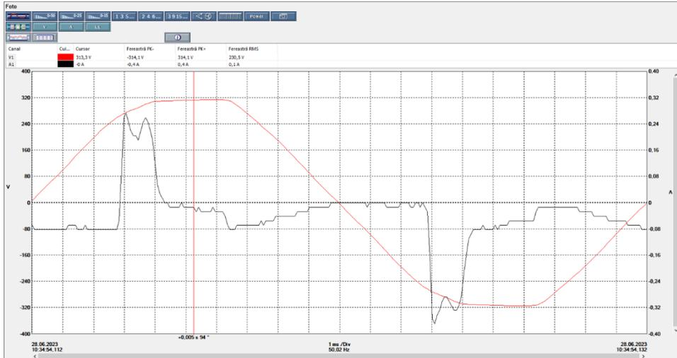
**Figure 6.** Voltage and current waveforms when operating 2 bulb-type LED sources.
