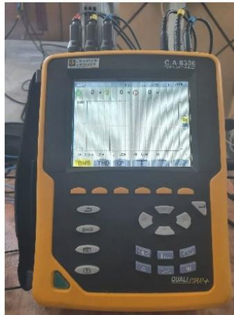
**Figure 2.** Network analyzer.
