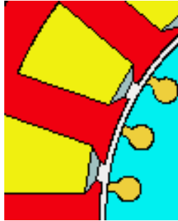
Figure 4. Shape of teeth and notches at the analyzed induction motor - modified rotor geometry
