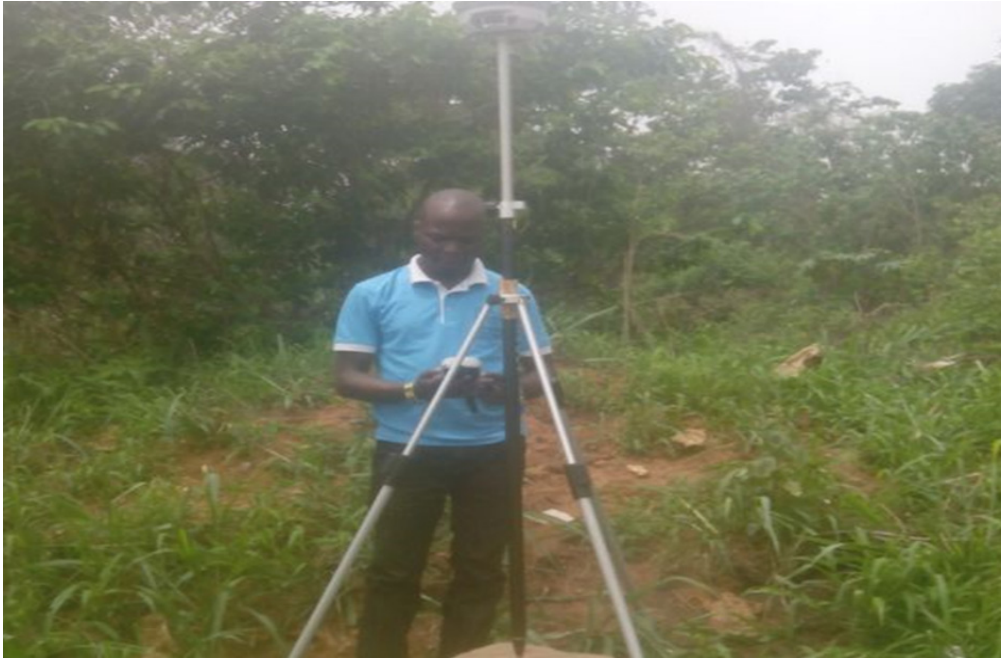
Figure 2. Hi-Target instrument set-up on one of the stations
