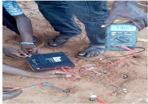
Figure 2. Testing of probe sensor electromagnetic flux at preset soil depth
