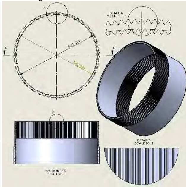
Figure 5. The geometry of the flexible wheel
