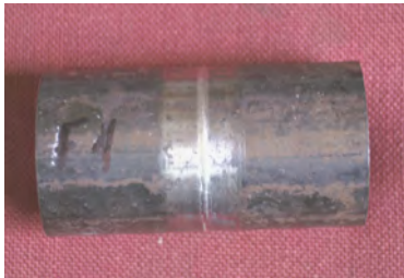
Figure 1. F1 butt welded sample, not heat treated.
