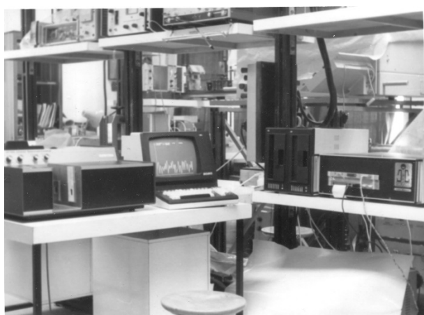
Figure 24. Unicam SP1100 Infrared Spectrophotometer with analog to digital conversion and 8080 processor as core of the computing system
