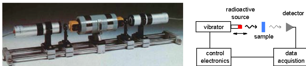
Figure 21. The radioactive source, electromagnetic drive to control the speed, the sample holder and the photomultiplier as a detector in a complete MS with a block schematic
