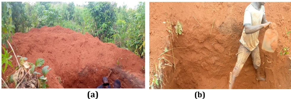
Figure 2. Excavating one of the pits to obtain soil samples from various profile depths
