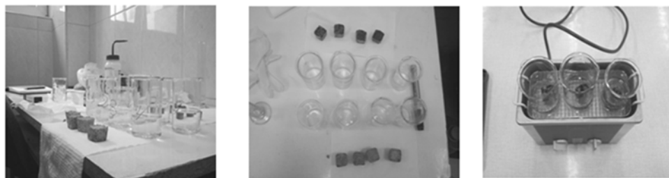
Fig. 1. Preparation for the ultrasonication and the ultrasonic bath S 10 H Elmasonic
