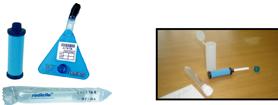
Fig. 4. Radiello passive samplers, blue diffusive body code 120-1 and supporting plate.
