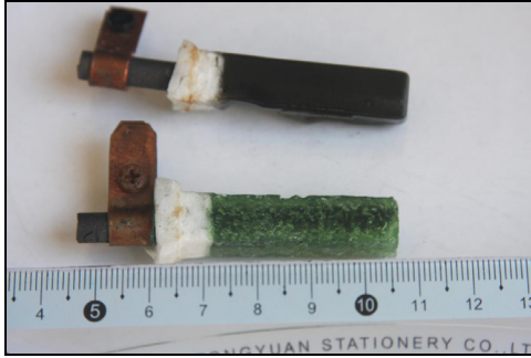
Fig. 2. The bacteria from sludge (up), and cyanobacteria (down) immobilized onto the electrodes.
