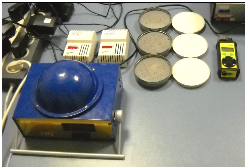
Fig. 1. The placement of the instruments at the 1st Intercomparison of continuous radon and its short-lived decay product monitors (NRPI, Prague) (RADIM 3A - left-down, DOSEMAN PRO - right top and the two RAMON 2.2 - center top).
