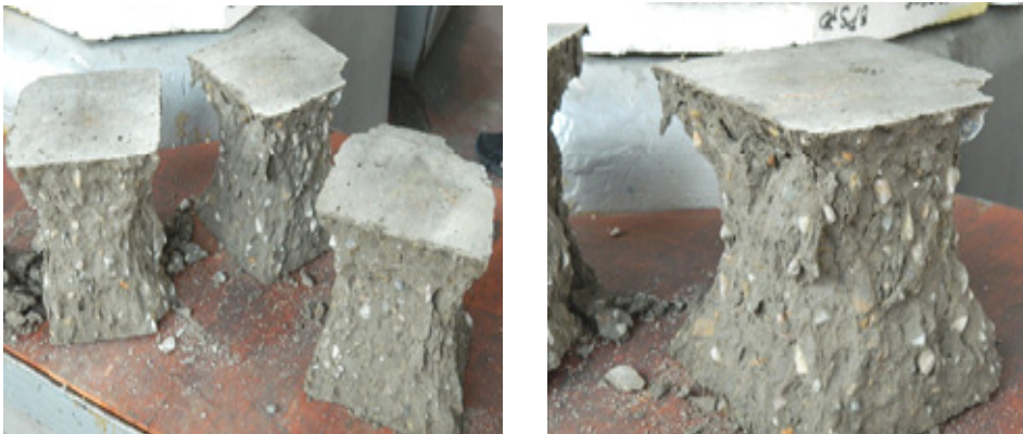
Fig. 10. Images of concrete with used sand subject to compression (casting 3)
