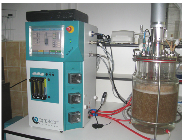
Fig. 1. Laboratory-scale bioreactor for submerged cultivation of edible and medicinal mushrooms
