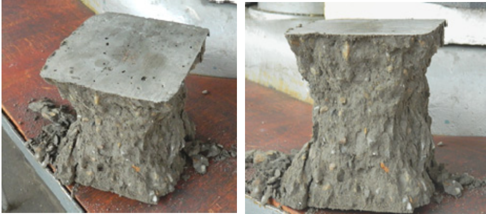
Fig. 9. Images of concrete with used sand, subject to compression testing (casting 2)
