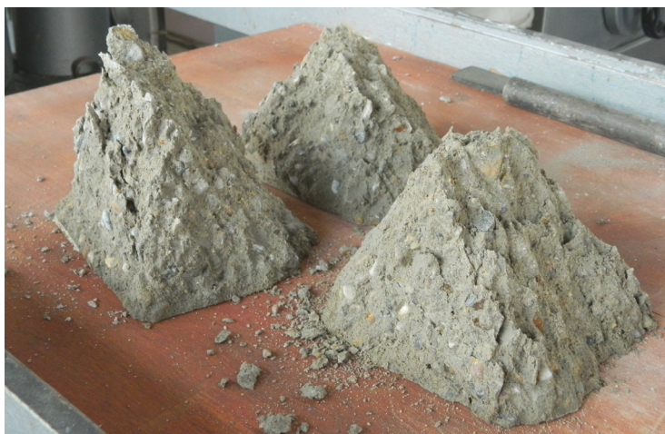
Fig. 8. Image of the concrete control casting subject to compression (casting 1)
