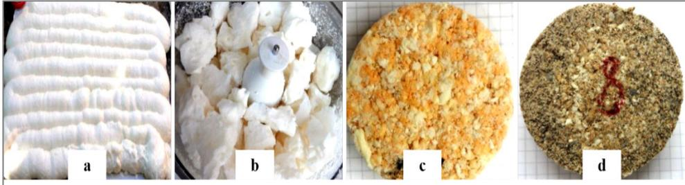
**Fig. 2.** *a. Waste from polyurethane foam. b. Material fragmentation. c. The hardened sample from the mixture of PU waste and PU adhesive. d. The hardened sample from the mixture of PU waste, PU adhesive and sand.*
