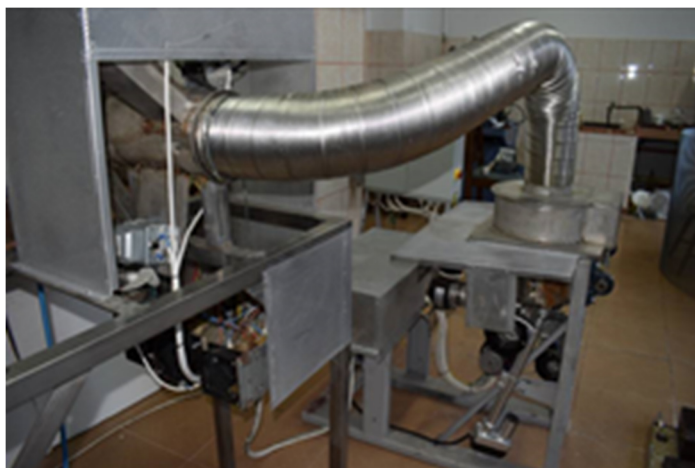
Fig. 2. Laboratory microwave furnace and gases thermal filter installation
