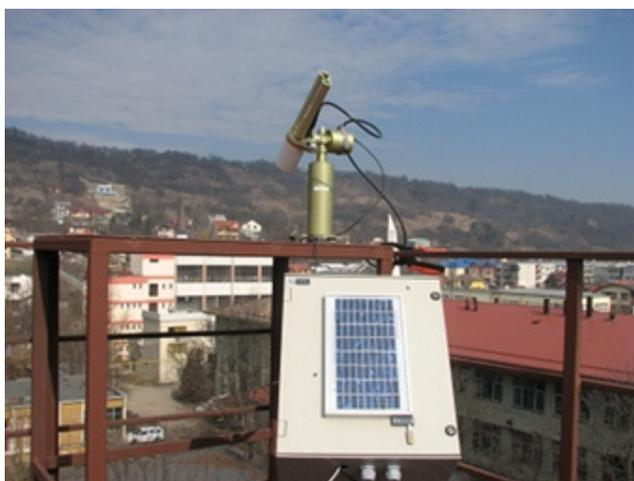
**Fig. 1.** CLUJ\_UBB site AERONET sun-photometer
