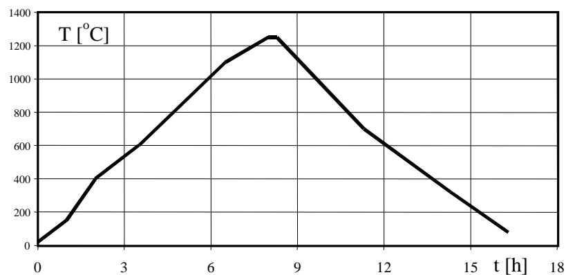
Fig. 2. Heating diagram for phosphatic porcelain.
