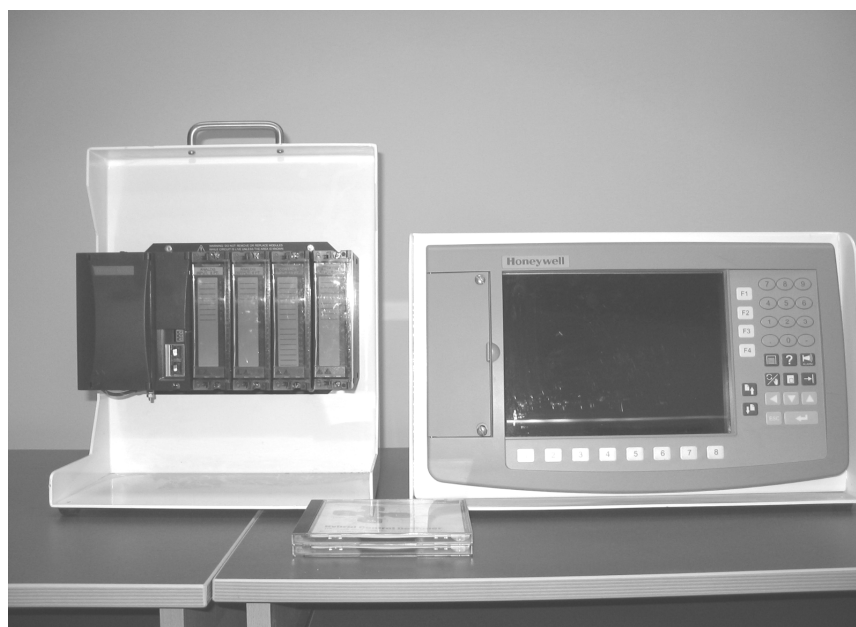
Figure 5. HC900 distributed system (Honeywell).
