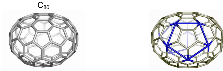
Figure 5. Retro-Quadrupling RQ operation on a pentagonal face
