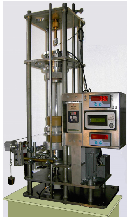
Figure 3a, b. The torsion measurement of the outer cylinder.
