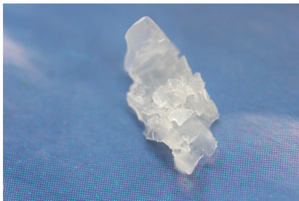
Figure 8. Photo of the gel obtained by linking P((EO)_2MA)-b-PIB-b-P((EO)_2MA) block copolymers via ATRP of EGDMA after purification.
