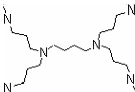
Figure 6. Polypropyleniminooctamin dendrimer NS_2[n] at generation n=1
