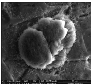
Figure 5b. Manganese dioxide germination on Ti–after S2 step; Electrolyte: 1\text{M H}_2\text{SO}_4 + 6\text{g/L Mn}^{2+} , \text{pH} \sim 0.5 , sweep rate 2\text{mVs}^{-1}
