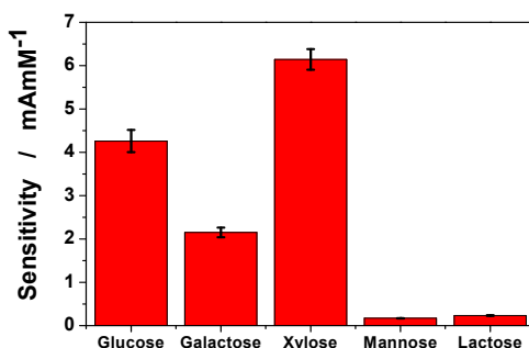
Figure 5. Sensitivity of G/Os-RP/dgPDH modified electrodes towards different substrates. The error bars correspond to the standard deviation for 3 successive measurements.
