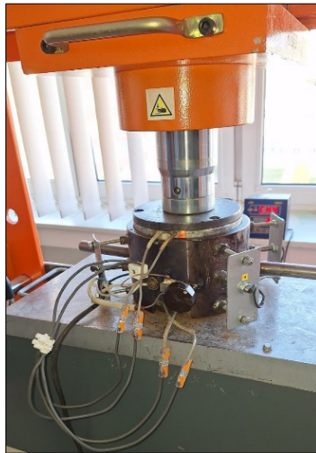
Figure 8. The mold used for the fabrication of composite plates.
