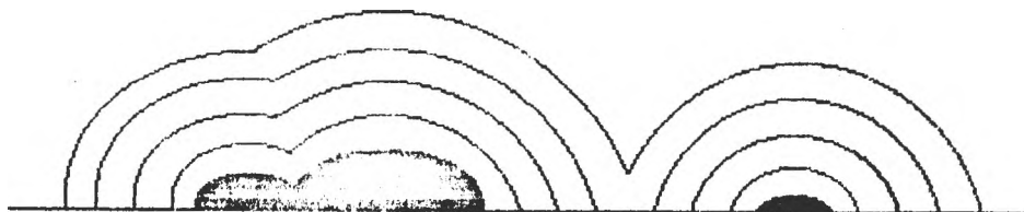
Figure1. Interference of the diffusion zones and overlap of the neighboring nuclei.
