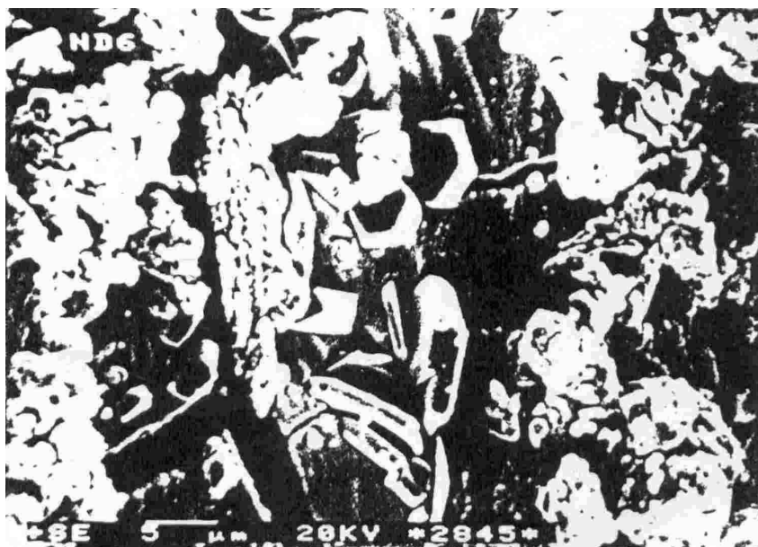
Fig. 4. SEM photograph of uncycled sintered cadmium electrode.
