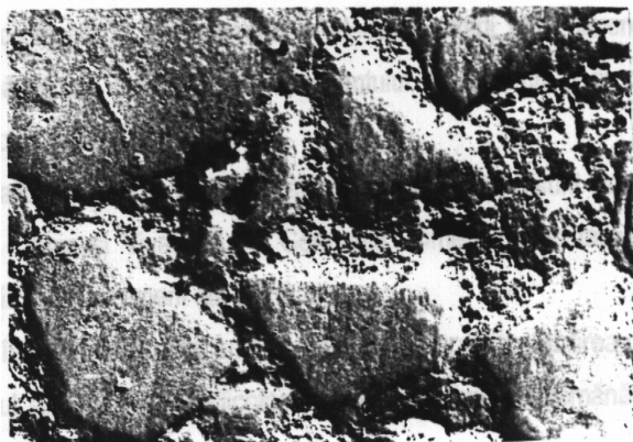
Figure 5. SEM image (x5000) of the ROMDENT zincophosphate cement hardened for 24 hours
