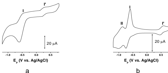
Fig. 5. Cyclic voltammograms of [\text{Bu}_4\text{N}]_{10}\text{H}_2[(\text{CeO})_3(\text{PW}_9\text{O}_{34})_2] (a) and [\text{Bu}_4\text{N}]_{10}\text{H}_2[(\text{CeO})_3(\text{AsW}_9\text{O}_{34})_2] (b) (0.1 M [\text{Bu}_4\text{N}]\text{ClO}_4 in acetonitrile, v = 100 \text{ mV s}^{-1} ).
