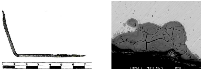
Figure 2. Bronze bended pin and SEM picture of the bronze artefact covered with a patina layer
