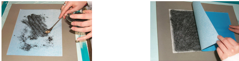
Figure 4. Manual doping of impregnated laminates.
