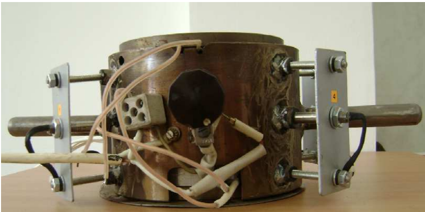
Figure 1. The plates fabrication mould.
