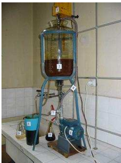
Figure 3. Pilot-equipment with magnetic separator (1-separator; 2- vessel with stirring; 3-stirrer; 4-recirculation pump; 5- tank for MF; 6- collecting vessel).
