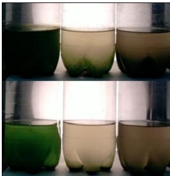
Figure 2. Top part: the result of the cessation of the carbon dioxide feed; Bottom part: the result of flow choke with carbon dioxide
