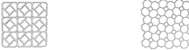
Figure 1. The 2-dimensional ((4,7)3) net (3×3 units) designed by the sequence of map operations Trs(Ca(4,4)) : non-optimized (left) and optimized (right) structure.
