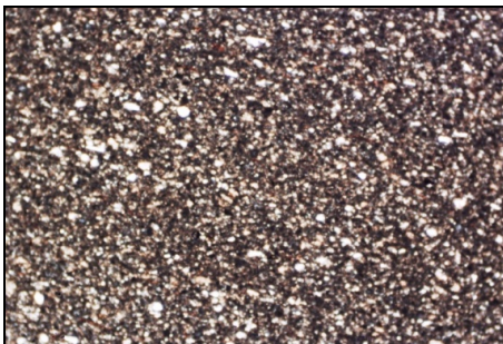
Figure 2. Electrotechnical porcelain with fine texture consisting of one vitreous and one crystalline phase; quartz is the dominant phase (1N)
