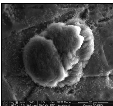
Figure 5b. Manganese dioxide germination on Ti–after S2 step; Electrolyte: 1M \text{H}_2\text{SO}_4 + 6g/L \text{Mn}^{2+} , pH \approx 0.5, sweep rate 2mVs ^{-1}
