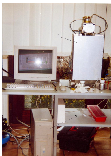
Figure 5. The stand with FIA 100: 1 - the apparatus FIA100; 2 - PC unit for data recording.
