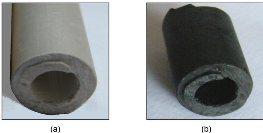
**Figure 2.** Blank  $\text{TiO}_2\text{-ZrO}_2$  (a) and  $\text{CX/TiO}_2\text{-ZrO}_2$  (b).
