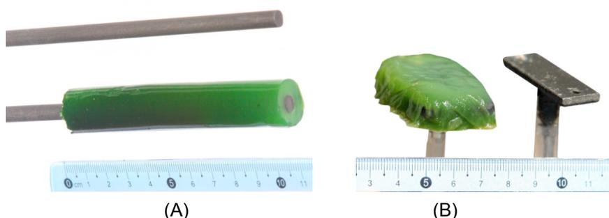
**Figure 6.** Image of the immobilized *Synechocystis* cathode and the control cathode (A) for two-chamber (B) for membraneless MFC.
