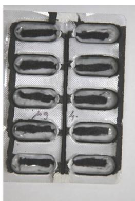
**Figure 9.** Blister of ten batteries ready for filling
