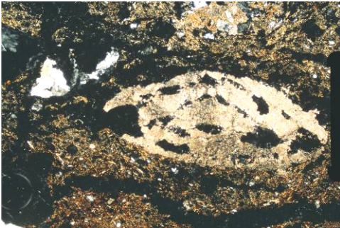
Fig.11. Sample 36 – Semifine to coarse ceramics with microcrystalline - amorphous matrix; quartz, micas, plagioclase feldspars, ceramoclasts, bioclasts (foraminifera and algae), iron oxy-hydroxide clusters, and limestone lithoclasts; N+, scale bar = 0.5 mm
