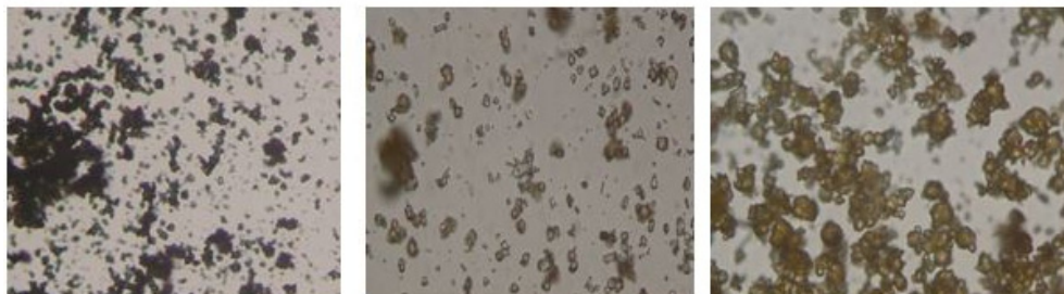
Figure 1. SEM micrographs of spray dried coffee sample
